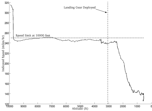
Figure 6: For the high airspeed anomaly the top anomalous parameter (airspeed) is plotted against altitude. The speed limit threshold at 10,000 ft. is denoted by the dashed line at 250 knots.
