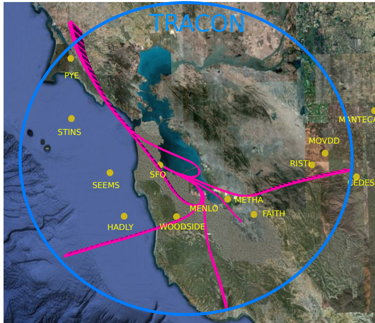
Figure 18. Centroids of the clusters and reporting points/way-points for SFO arrivals. Those centroids differ from the ones in Figure 13 because the algorithm was run with different parameters with a smaller sensitivity.
