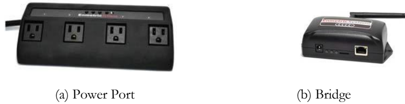
Figure 2 Plug load management equipment.
