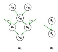
Fig. 3. The part of the BN corresponding to (a) a relay and (b) a current sensor.
