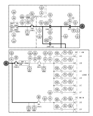
Fig. 1. Schematic of the ADAPT testbed, showing one of three power storage parts (for Battery 1, top) and one of two load banks (Load bank 1, bottom). Detailed information about loads is given in Table II.
