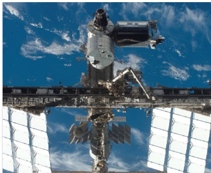
Figure 5. ISS external view showing ETCS radiators at lower left and lower right.
