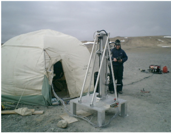
Figure 2: DAME Mars Drill System
