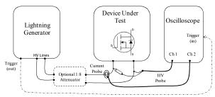
Figure 5. Pin injection test setup diagram.
