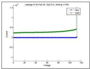
Figure 9. Drain-to-source leakage current plot for G-S injection at high voltage setting (76V).
