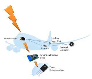
Figure 2. Propagation of lightning event through avionics.
