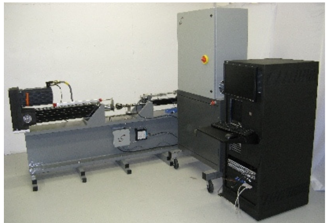
Figure 6 – New EMA test stand at NASA Ames research center.
