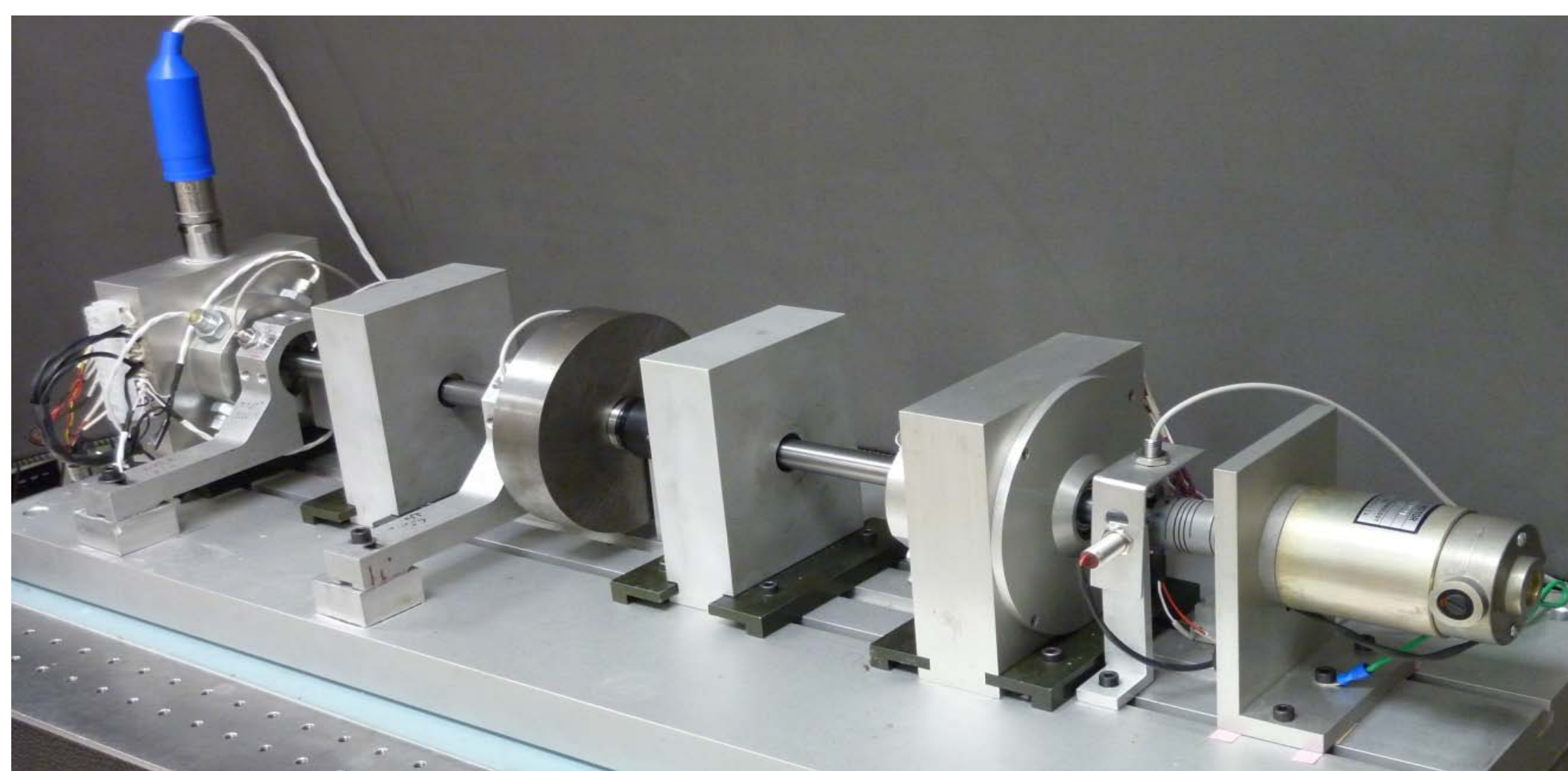
Experimental Crack Detection Test Rig
