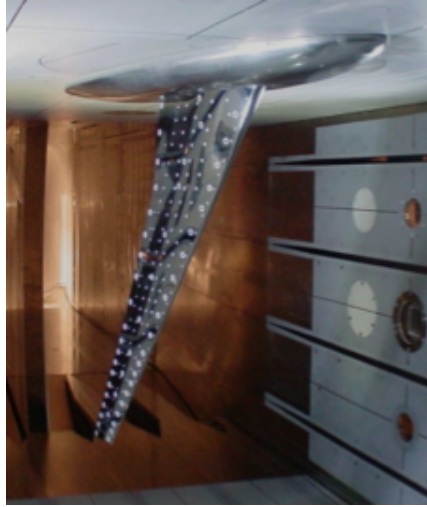
Fig. 2: HIRENASD mounted in wind-tunnel
