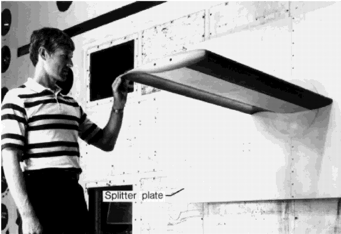
Figure 1. Rectangular supercritical wing installed in wind tunnel.
